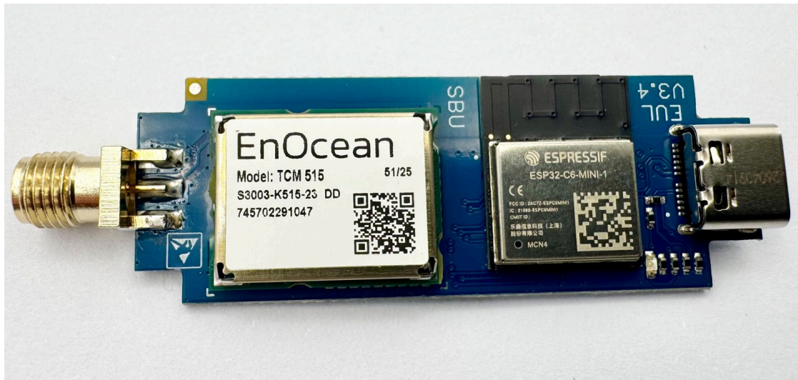
EUL32, circuit board V3.4: RP-SMA socket, EnOcean TCM 515, ESP32-C6-MINI-1, USB-C
