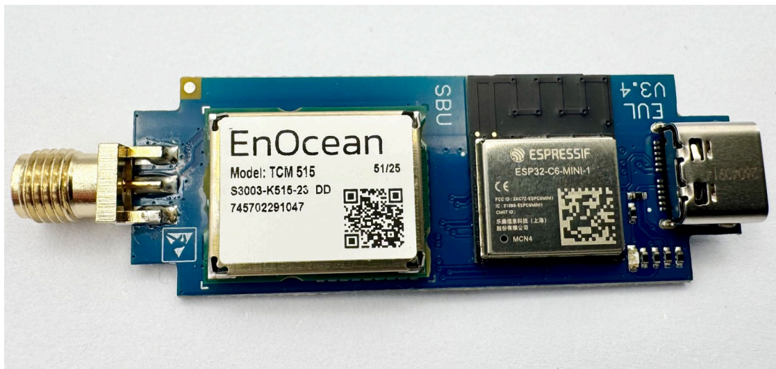
EUL32, Leiterplatte V3.4: RP-SMA-Buchse, EnOcean TCM 515, ESP32-C6-MINI-1, USB-C
